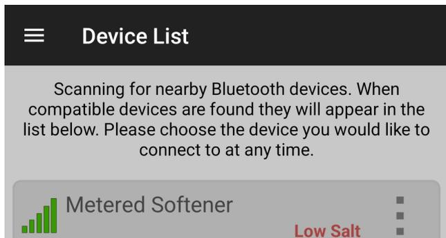
When a valve reports it has low salt it can be seen on the device list when you initially open the app. This happens when the salt level in the brine tank is determined to be at 20% or less.
