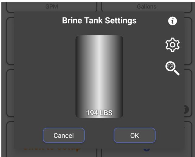
Once the initial configuration is complete you can enter the current salt level in the tank by either tapping the brine tank or sliding up and down to the desired position. This will need updated every time you add salt to your brine tank. You can also adjust the initial configuration by tapping the gear icon and you can also configure the salt monitoring by clicking the magnifying glass icon (specific instructions about this later in the “Salt Monitoring” section).
