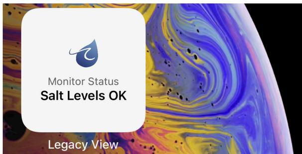
Once setup, the widget will trigger a Bluetooth scan every 30 minutes, as mentioned above. If all softeners are reporting as having adequate salt levels, then it will display “Salt Level OK”. If a softener is reporting that it has low salt, then “Salt Level Low” will be displayed. Once you add more salt to your brine tank and adjust the level in the app it will report adequate again. Tapping this widget will also open the app.
