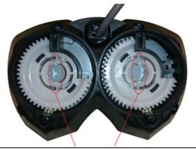
When reinstalling the motorized bypass, make sure that that the orientation of the clips on the handles match the grooves on the valve stems where the motorized bypass drive was removed.
