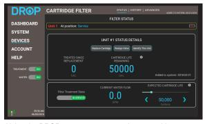
Using the DROP app on your smart phone or tablet, connect to your DROP system. On the navigation menu on the left choose "Devices", and then choose your Cartridge Filter from that list. Assuming you have one filter, you will see a "Replace Cartridge" button on the screen. Press that button and the lights on the cartridge filter should turn yellow. Wait until the lights stop spinning before going to the next step (Should take approximately 30 seconds and you should hear the motors turning).
